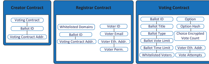
Fig. 1. Memory field structure of smart contracts in GenVote, where lines between fields represent relational data [8].
