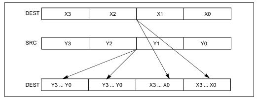
Figure 3-17. SHUFPS Shuffle Operation
