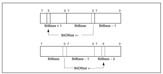
Figure 3-2. Memory Bit Indexing
