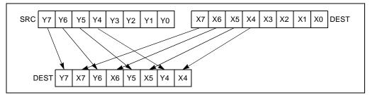
Figure 3-14. PUNPCKHBW Instruction Operation Using 64-bit Operands
