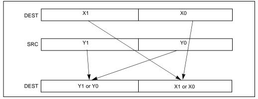
Figure 3-16. SHUFPD Shuffle Operation
