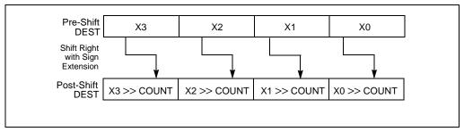
Figure 3-12. PSRAW and PSRAD Instruction Operation Using a 64-bit Operand
