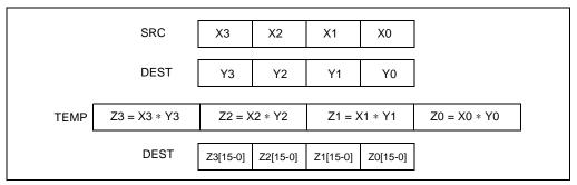
Figure 3-8. PMULLU Instruction Operation Using 64-bit Operands
