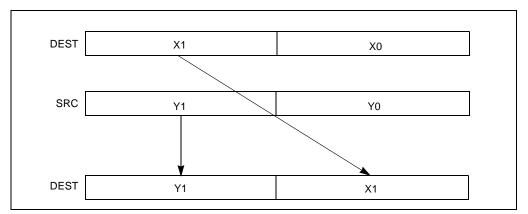
Figure 3-18. UNPCKHPD Instruction High Unpack and Interleave Operation
