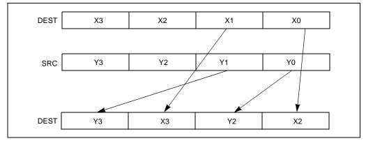
Figure 3-21. UNPCKLPS Instruction Low Unpack and Interleave Operation
