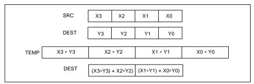
Figure 3-6. PMADDWD Execution Model Using 64-bit Operands
