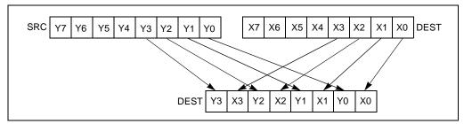
Figure 3-15. PUNPCKLBW Instruction Operation Using 64-bit Operands
