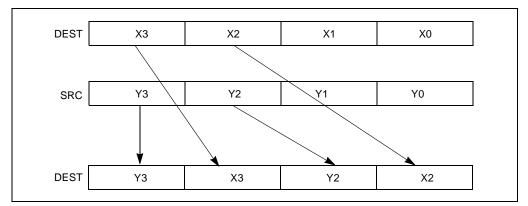
Figure 3-19. UNPCKHPS Instruction High Unpack and Interleave Operation
