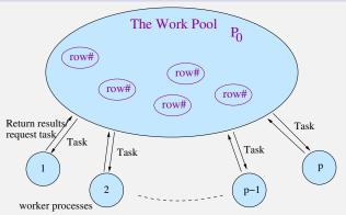
The work pool holds a collection of tasks to be performed. Processes are supplied with tasks as soon as they finish previously assigned task. In more complex work pool problems, processes may even generate new tasks to be added to the work pool.
