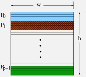
The display width = w, and the display height = h. Each process handles at most  $\lceil h/p \rceil$  rows. Total number of points  $= n = h \times w$ .
