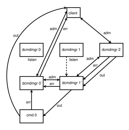
Figure 4.6.: The fully connected tail dcmdmgr creates a pipe to receive error messages from its child. When the command is fork()-ed and exec()-ed, its stdout, stdin, and stderr are assigned to the sockets and pipe established by its parent. While this is happening, the second dcmdmgr is establishing connections to its upstream dcmdmgr.
