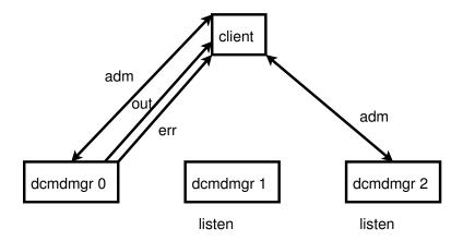
Figure 4.4.: As the furthest downstream process, the client initiates pipeline establishment by connecting to the tail dcmdmgr.
