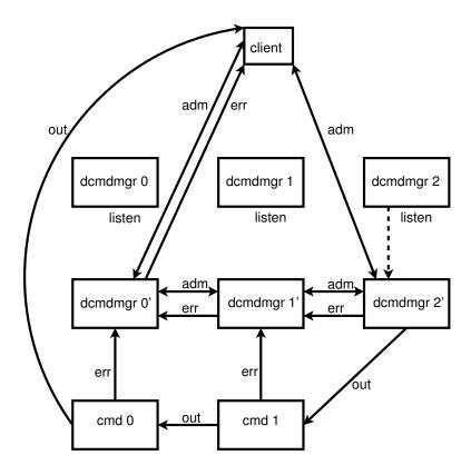
Figure 4.7.: The second dcmdmgr fork()s and exec()s its command. The head dcmdmgr has no upstream dcmdmgr and already has its "upstream" administrative socket. It is fully connected and ready to fork() and exec() its own command.
