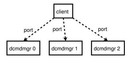
Figure 4.1. The client starts one dcmdmgr on each selected node.
