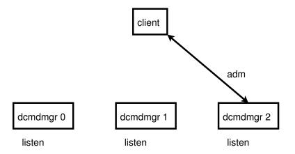
Figure 4.3.: All dcmdmgrs listen for administrative, error, and output socket connections from downstream.
