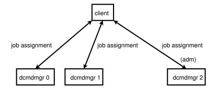
Figure 4.2.: The client sends each dcmdmgr its job assignment. Assignment order is from tail to head with the head dcmdmgr retaining the socket as its upstream administrative socket.
