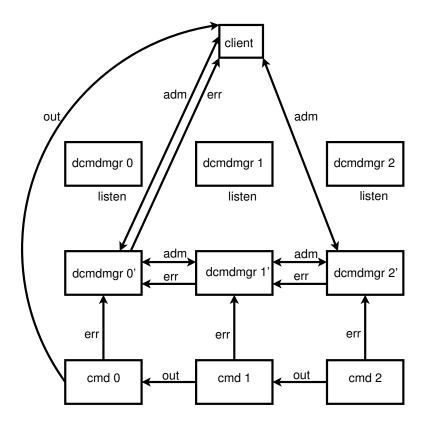
Figure 4.8.: When the head dcmdmgr has fork()-ed and exec()-ed its command, the process pipeline and parallel dcmdmgr pipelines are fully connected and operational. All top-level dcmdmgrs are free to listen for their next job assignments.
