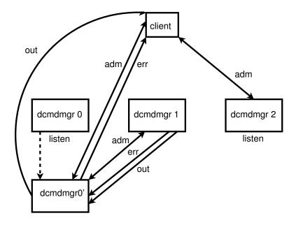
Figure 4.5.: The downstream-connected tail dcmdmgr fork()s a child to contact its upstream dcmdmgr which may be the parent or a dcmdmgr on another node.
