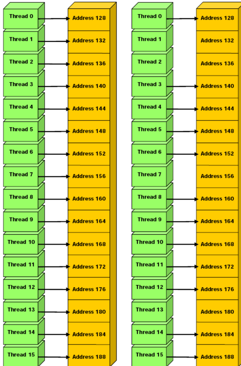
Figure 3.8: Examples of coalesced global memory access patterns (courtesy of NVIDIA). Left: coalesced float memory access, resulting in a single memory transaction. Right: coalesced float memory access (divergent warp), resulting in a single memory transaction.
