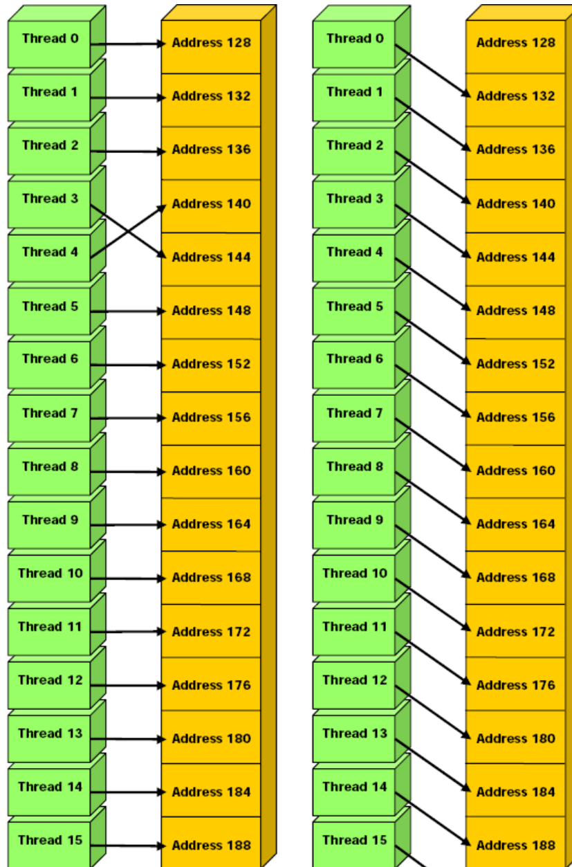
Figure 3.9: Examples of global memory access patterns that are non-coalesced for devices of compute capability 1.0 or 1.1 (courtesy of NVIDIA). Left: non-sequential float memory access, resulting in 16 memory transactions. Right: access with a misaligned starting address, resulting in 16 memory transactions.
